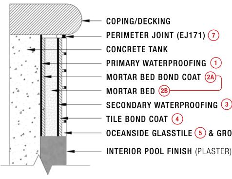
COPING/DECKING PERIMETER JOINT (EJ171) (7) **CONCRETE TANK** PRIMARY WATERPROOFING (1) MORTAR BED BOND COAT (2A) MORTAR BED (2B) SECONDARY WATERPROOFING (3) TILE BOND COAT (4) OCEANSIDE GLASSTILE (5) & GROUT (6)
